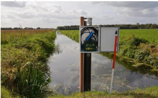
To identify the necessary measures, the quality of surface water is measured. Image: Pilot with online water quality measurement.
